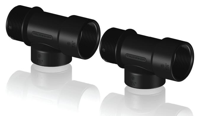
The T-Piece Threaded 11/2" BSP M-F-F is moulded from a glass-reinforced Nylon composite. High strength, highmodulus glass fibres provide dramatic strength, stiffness, toughness and dimensional stability. These are some of the unique properties that give significant advantages and weight-savings over traditional metallic fittings.
